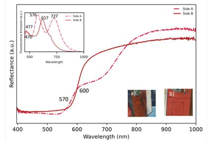
Fig.3.3. HSI reflectance and UV fluorescence spectra for the two red area on each side of the fan
