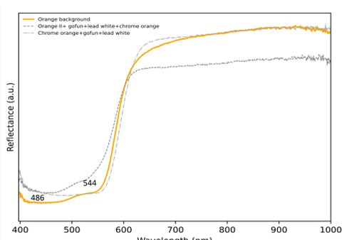
Fig.6.1. Reflectance spectrum of the orange background compared to some reference spectra of our database
