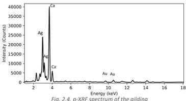
Fig. 2.4. p-XRF spectrum of the gilding
