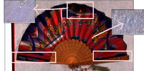
Fig.3.2. Image in false colour infrared (R=900nm; G= 650nm; B= 540nm) and with a dinolite® at x200 magnification
