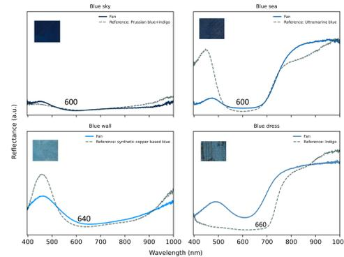
Fig. 3.1. HSI reflectance spectra of the 4 blue present on the fan compared to reference spectra.
