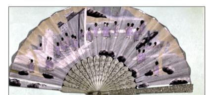
Fig.3.4. Image in false colour of the fan showing the different materials used. FC- R=2059nm; G=2202nm; B=2290 nm
