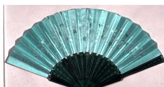
Fig.5.3. SWIR Image in FC with the characteristic bands of silk (R=2205nm; G=1575nm; B=1536nm)
