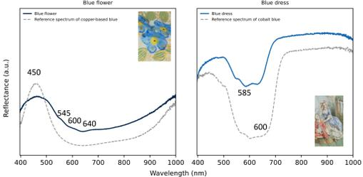
Fig. 2.1. a) HSI VIS reflectance spectra of two blue areas showing the use of two blue pigments.
